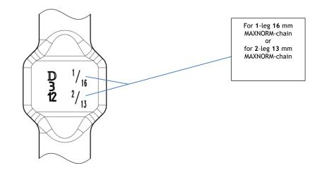
2.1 Assembly of the clevis head assembly system
