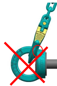
Fig. 4: A load of >90^\circ is not allowed if the hooked-in attachment device is supported on the load or on the ring point body.
