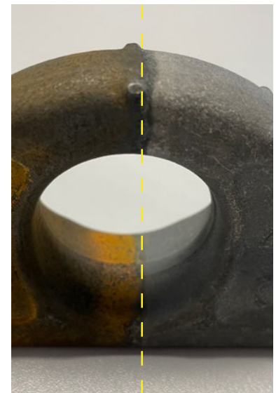
Without ZD (non corrosion protection)
