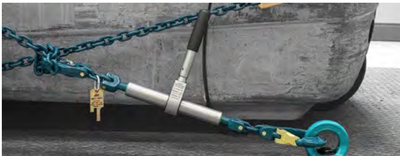
Variante 1 MAXNORM Zurrkette Variante 1 MAXNORM lashing chain
